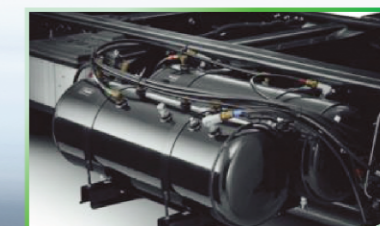
Phanh khí nén toàn phần (FVR/FVM/FVZ) Full-air brake with air dryer (FVR/FVM/FVZ)
