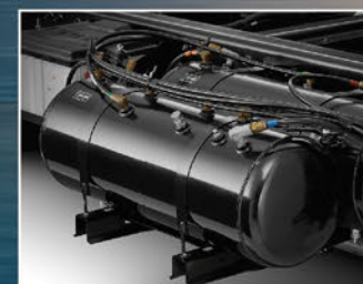
Phanh khí nén hoàn toàn (FVR & FVM) Full Air Brake with Air Dryer (FVR & FVM)
